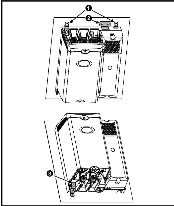
1. Common Unidrive SPM mounting bracket. Ensure short section attached to backplate
