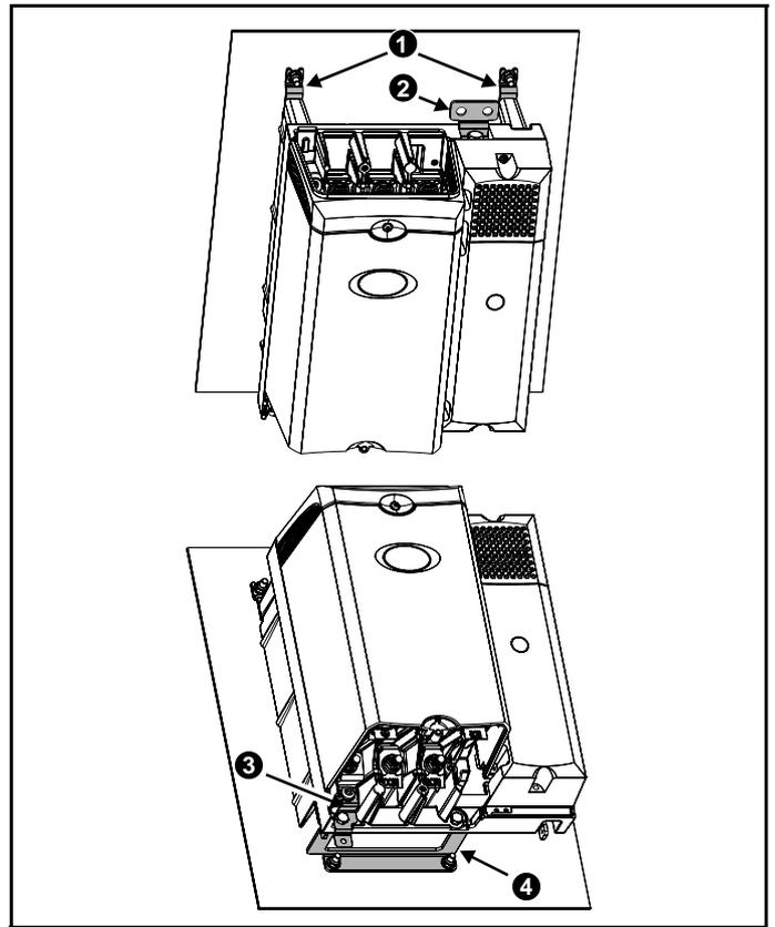
1. Common Unidrive SPM mounting bracket. Ensure short section attached to backplate
