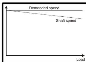
In order to prevent the speed droop shown above slip compensation should be enabled.
