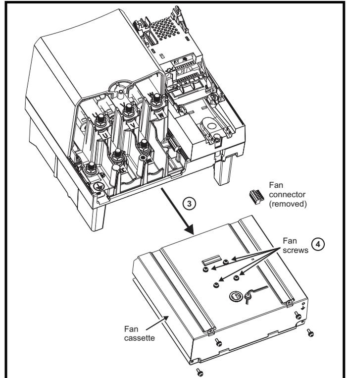
1. Remove the cable from the fan connector
