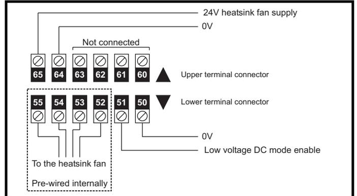
**Figure 6-39** SPMD low voltage DC mode enable connections
