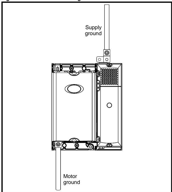
**Figure 6-6 Unidrive SPMD and SPMC/U (rectifier) ground connections**
