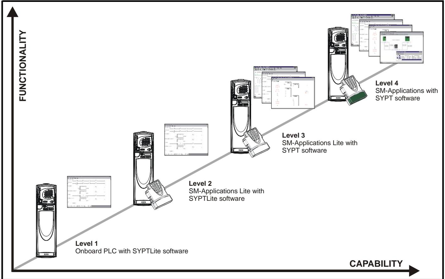
SYPTLite can be used with either the Onboard PLC in the Unidrive SPM or with SM-Applications Lite to create ladder logic programs.
