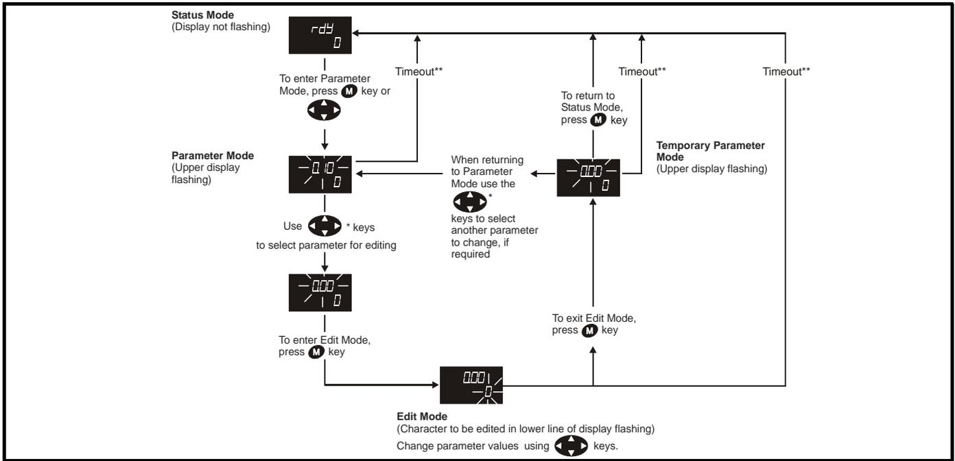
\* can only be used to move between menus if L2 access has been enabled (Pr 0.49). Refer to section 7.9 on page 84.
