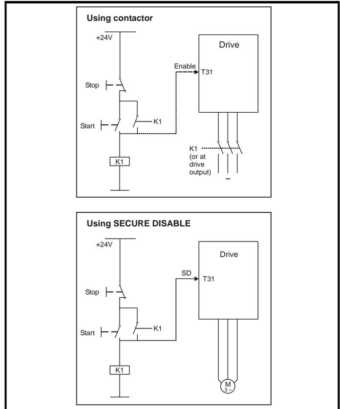
In the second example, illustrated in Figure 6-41 and Figure 6-42, a conventional high-integrity system which uses two safety contactors with auxiliary contacts with connected movement is replaced by a single Secure Disable system. This arrangement meets EN954-1 category 3.
