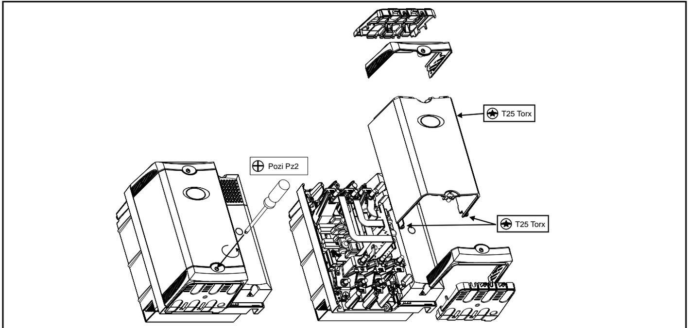
When removing the Unidrive SPMC/U dual rectifier centre housing, undo the 3 x T25 torx head screws as shown in Figure 5-3. When the housing is replaced, the screws should be tightened with a maximum torque of 2.5 N m (1.8 lb ft).
