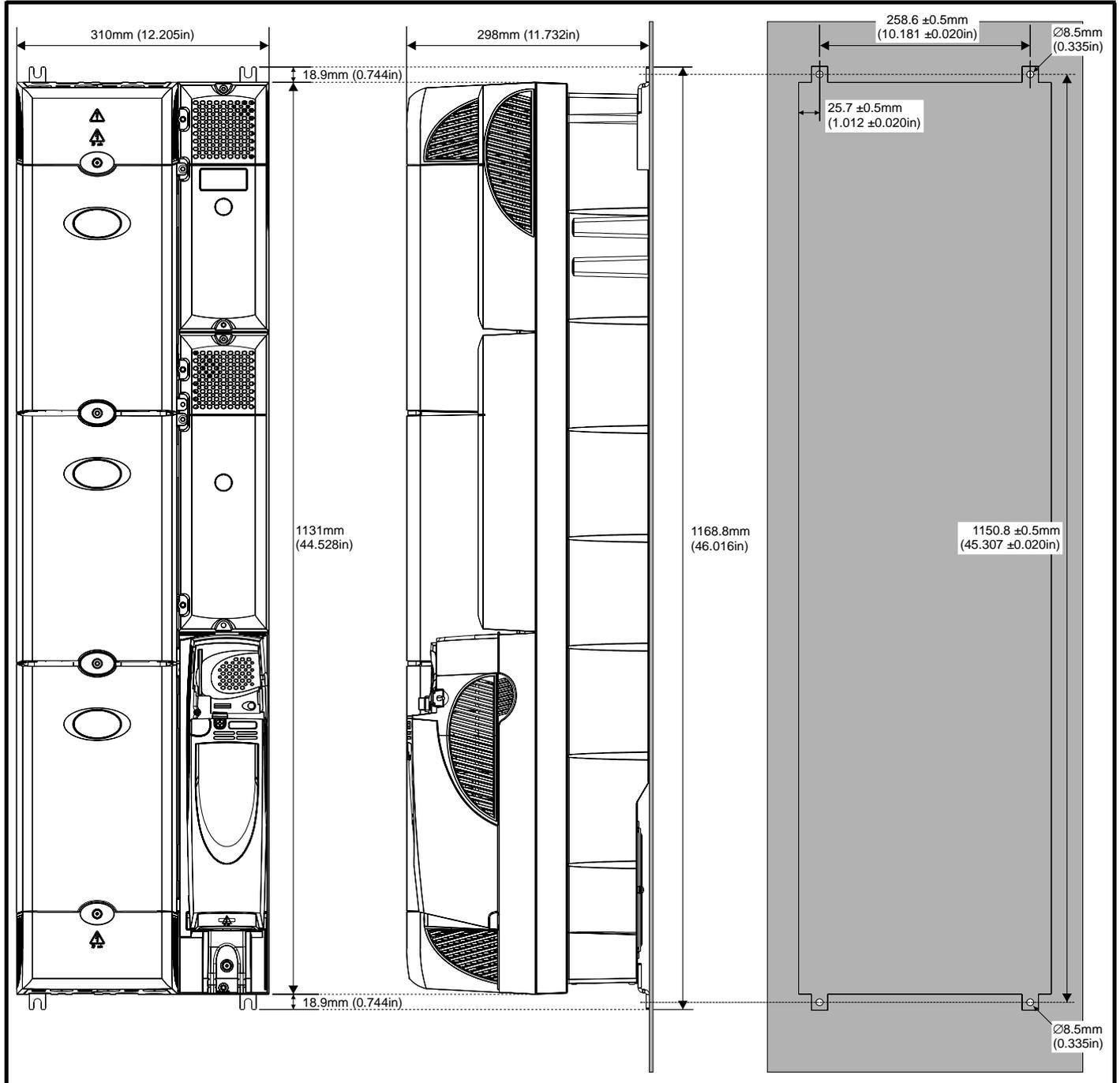
**Figure 5-8 Surface mounting the Unidrive SPMD**
