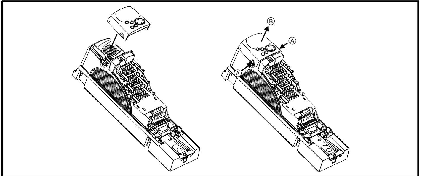
To fit, align the keypad and press gently in the direction shown until it clicks into position.
