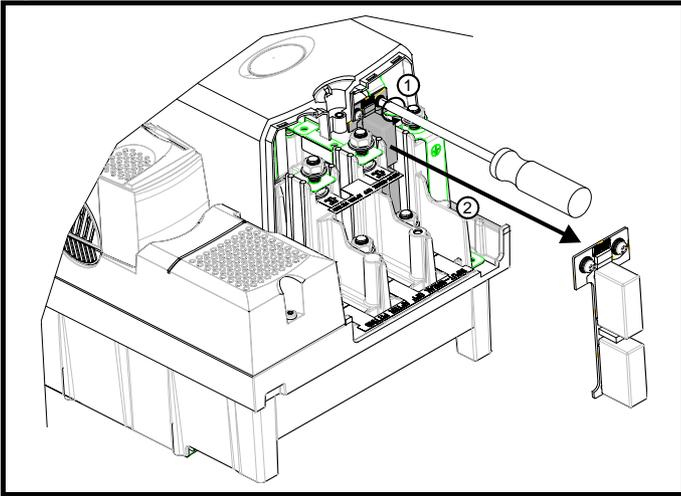
Loosen screws (1). Remove EMC filter in the direction shown (2).
