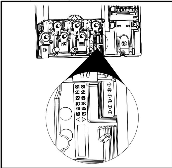
**Figure 6-9 Heatsink fan supply connections (SPMA & SPMD)**
