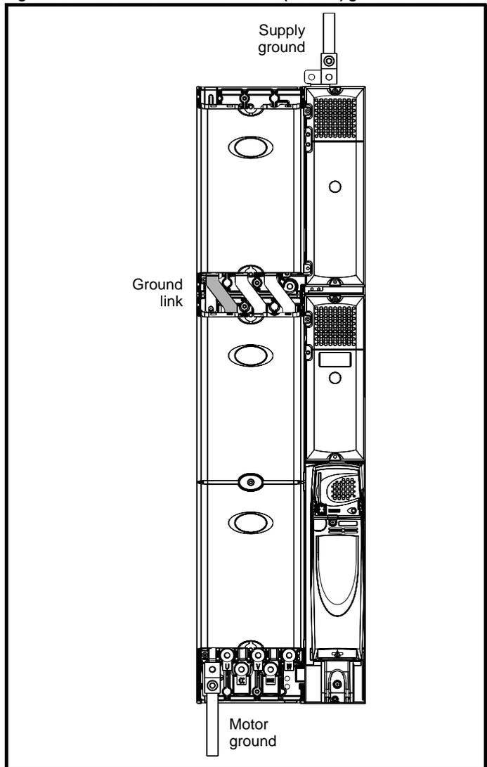
**WARNING** The ground loop impedance must conform to the requirements of local safety regulations.
