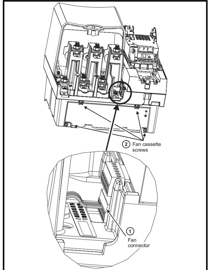
Figure 5-26 Removing the fan part 2
