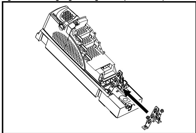
Loosen the ground connection nuts and slide the grounding bracket in the direction shown. Once in place, re-tighten the ground connection nuts.
