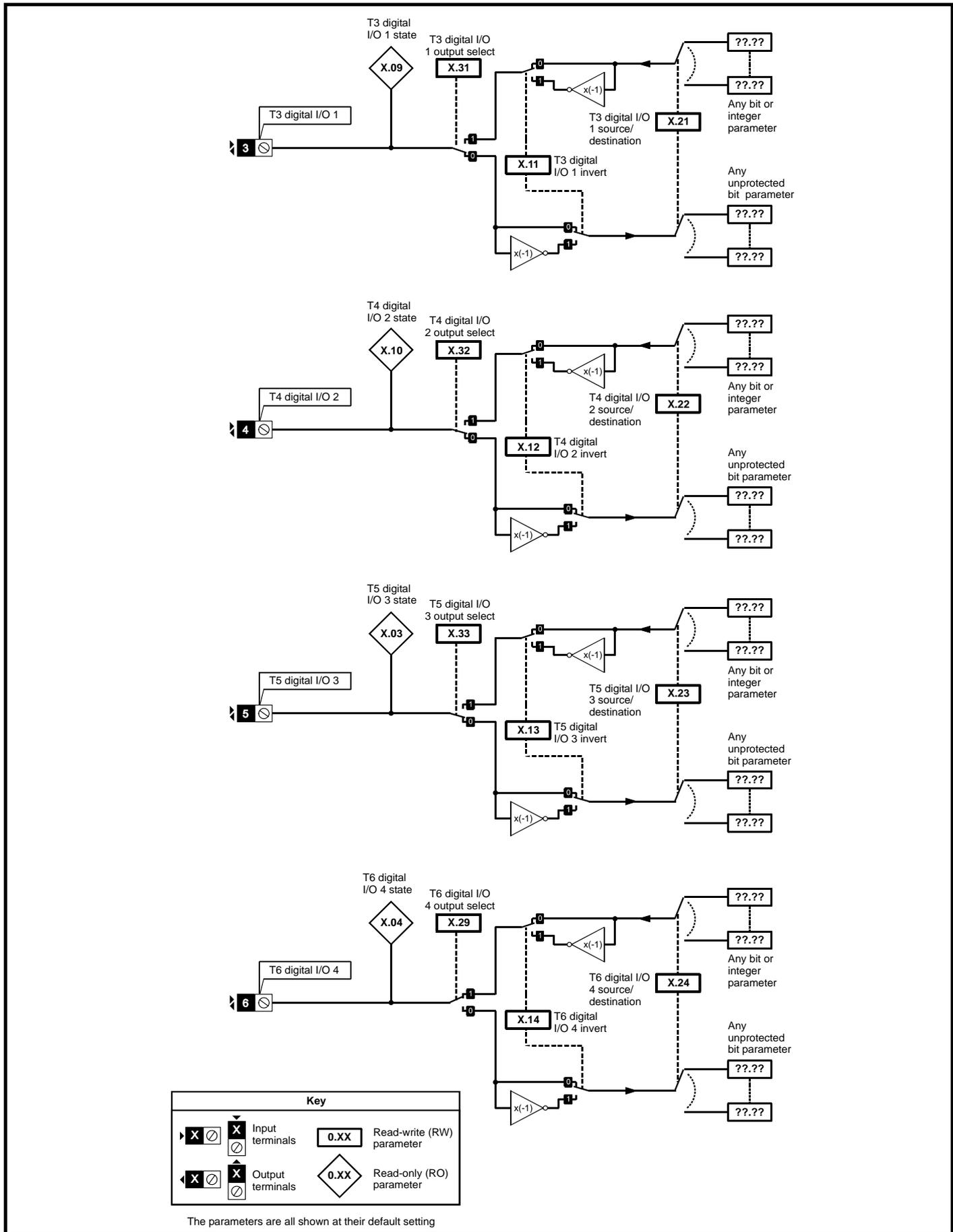
**Figure 13-34 SM-PELV digital input logic diagram**
