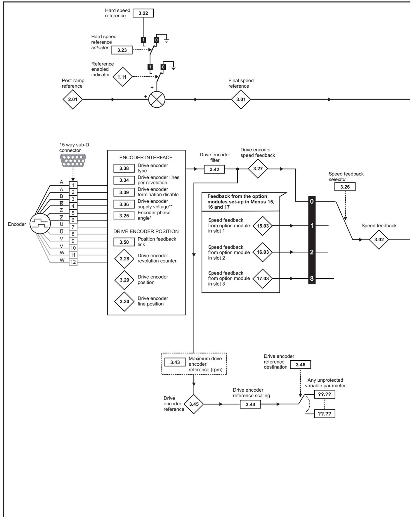
**NOTE** \*\*If Ab encoder voltage is greater than 5V, then the termination resistors must be disabled Pr 3.39 to 0.
