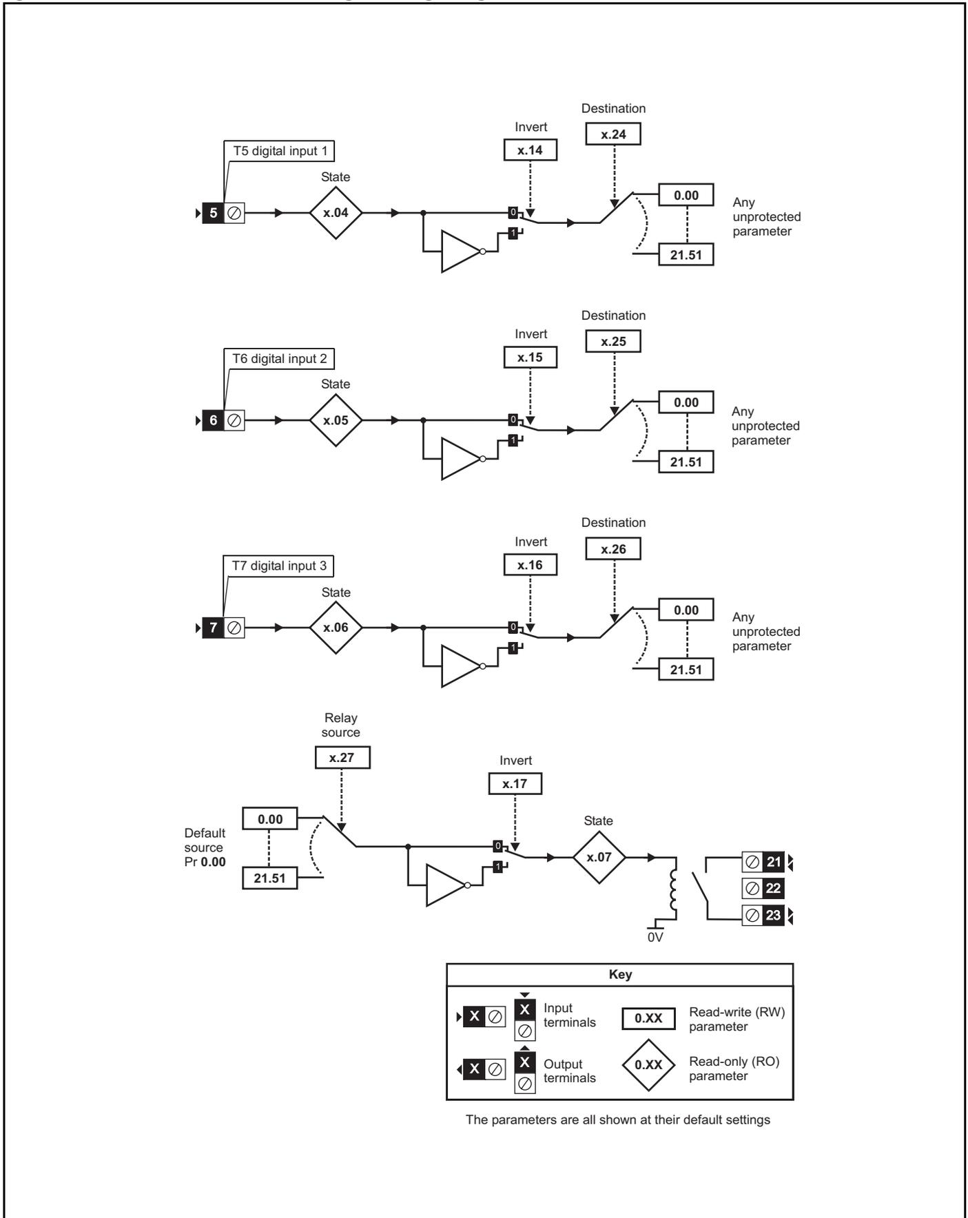
**Figure 13-31 SM-I/O Lite & SM-I/O Timer analogue I/O logic diagram**
