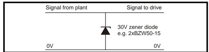
**Figure 6-30 Surge suppression for analogue and bipolar inputs and outputs**
