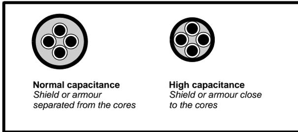
The cable used for Table 6-14 and Table 6-15 is shielded and contains four cores. Typical capacitance for this type of cable is 130pF/m (i.e. from one core to all others and the shield connected together).
