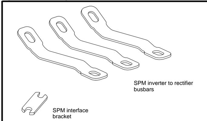
The SPM interface bracket should be connected first, followed by the SPM inverter to rectifier busbars, to the appropriate terminals as shown in Figure 5-21.
