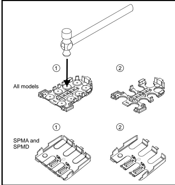
Place finger-guard on a flat solid surface and hit relevant break-outs with hammer as shown (1). Continue until all required break-outs are removed (2). Remove any flash / sharp edges once the break-outs are removed.
