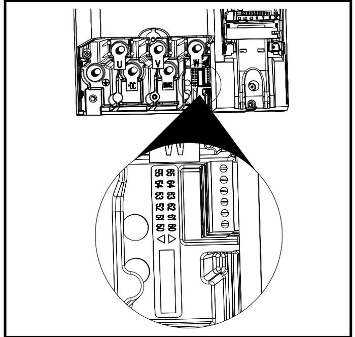
**Figure 6-38** SPMA low voltage DC mode enable connections
