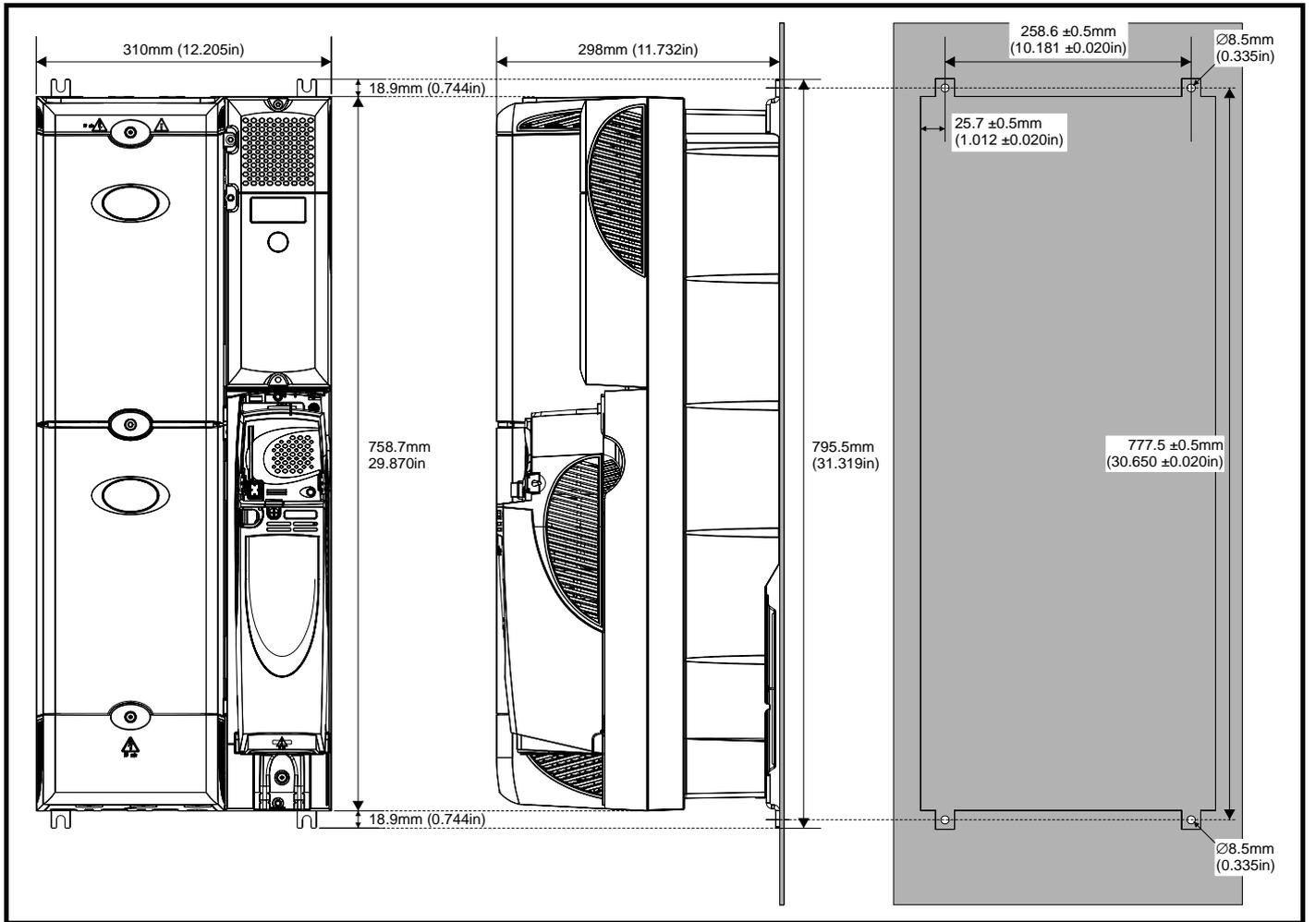
**Figure 5-9 Surface mounting the Unidrive SPMC/U (rectifier)**
