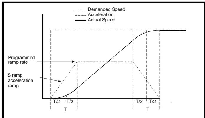
Since the ramp rate is defined in s/100Hz or s/1000rpm and the S ramp parameter is defined in s<sup>2</sup>/100Hz or s<sup>2</sup>/1000rpm, the time T for the 'curved' part of the S can be determined from:
