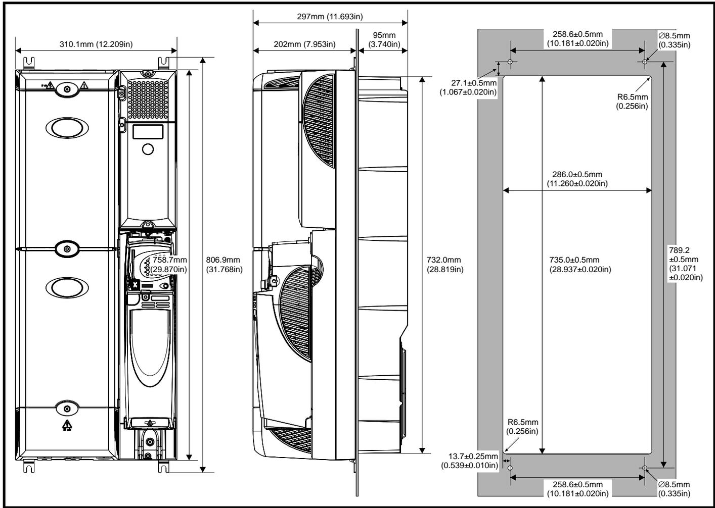
**Figure 5-13 Through-panel mounting the Unidrive SPMC/U (rectifier)**
