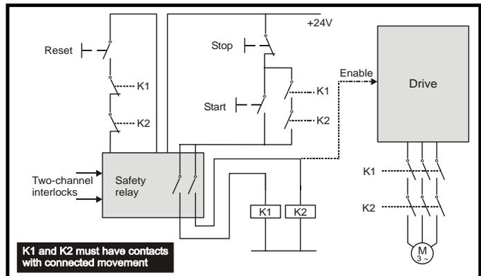
The safety function of the example circuit is to ensure that the motor does not operate when the interlocks are not signalling a safe state. The safety relay is used to check the two interlock channels and detect faults in those channels. The stop/start buttons are shown for completeness as part of a typical arrangement, they do not carry out a safety function and
