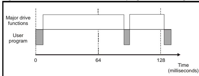
The user program is scheduled for a short period approximately once every 64ms. The time for which the program is scheduled will vary between 0.2ms and 2ms depending on the loading of the drive's processor.
