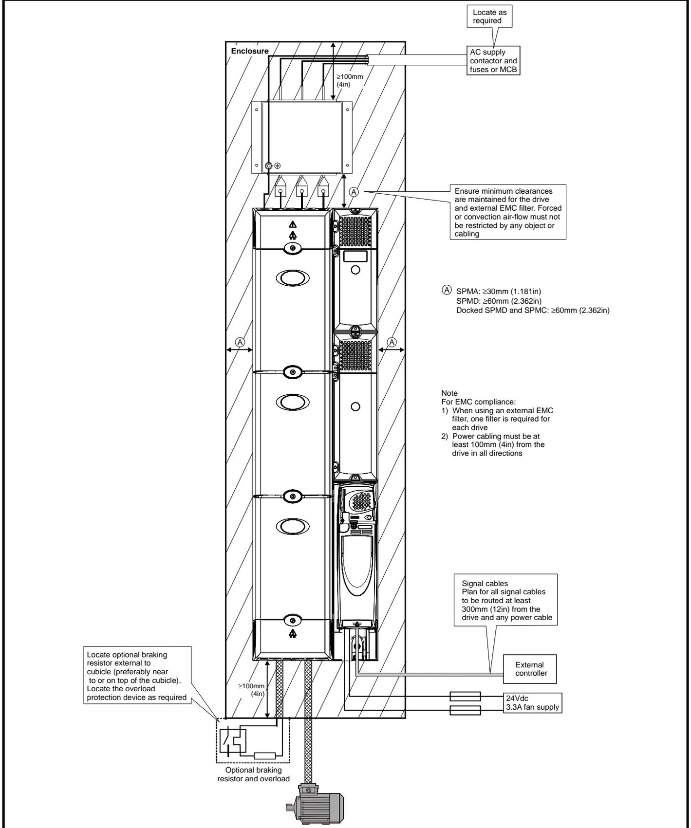
Figure 5-23 Alternative enclosure layout: Undocked Undrive SPMD and SPMC
