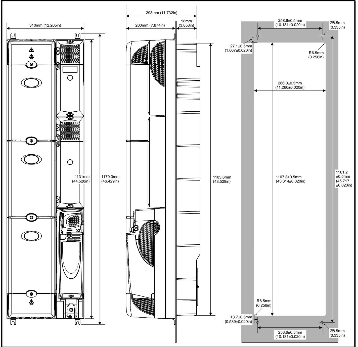
**Figure 5-12 Through-panel mounting the Unidrive SPMD**
