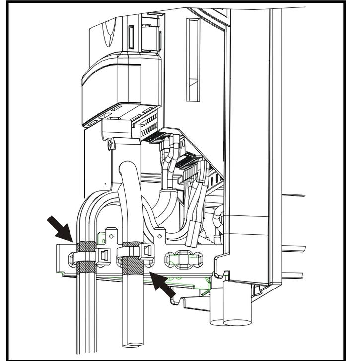
**Figure 6-26 Grounding of SPMC/U signal cables**
