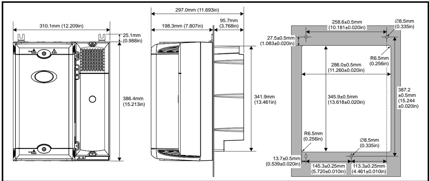
**Figure 5-14 Through-panel mounting the Unidrive SPMD with SPMC/U (rectifier) and docking kit**
