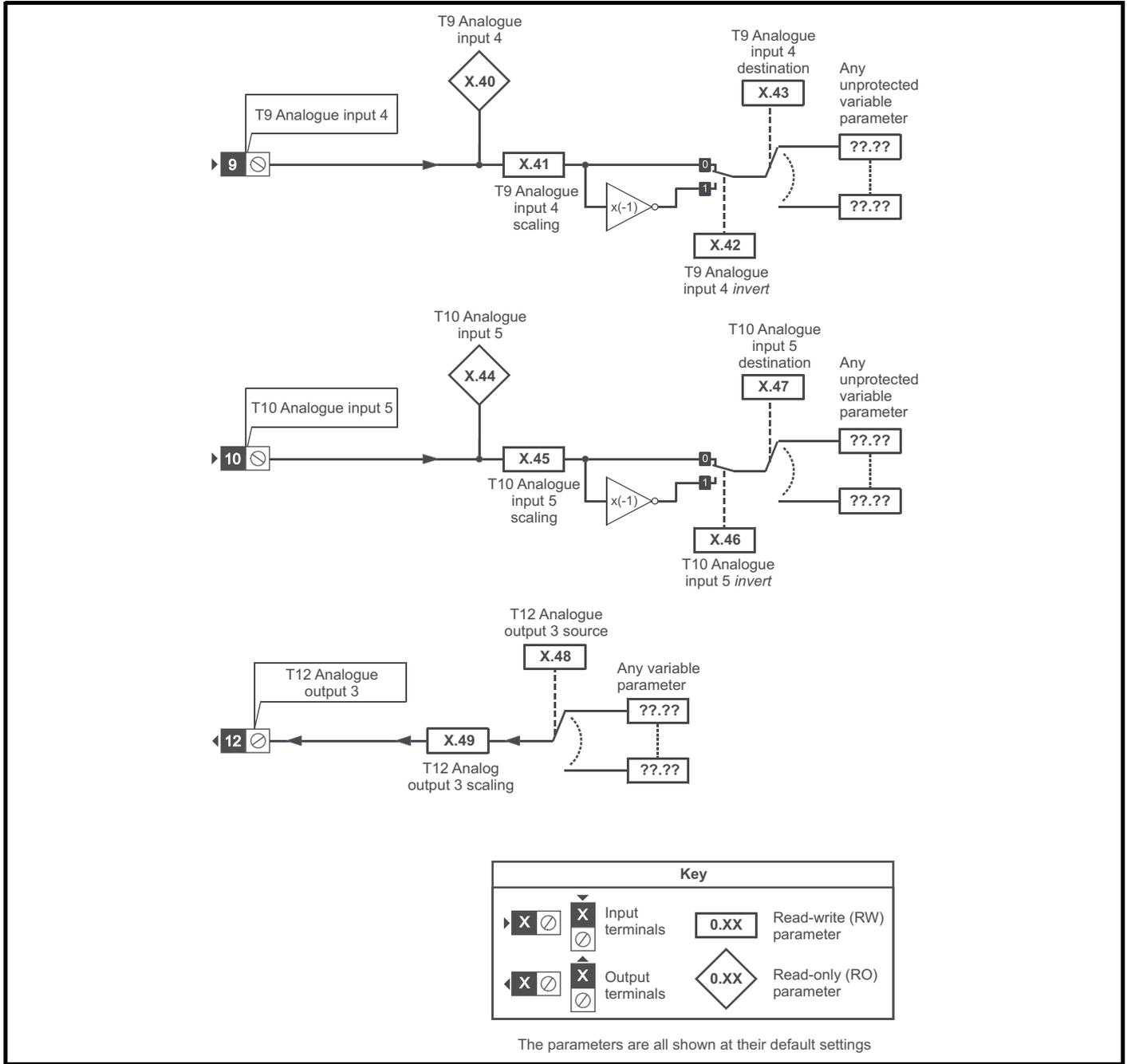
Figure 13-28 SM-I/O Plus digital logic diagram 1
