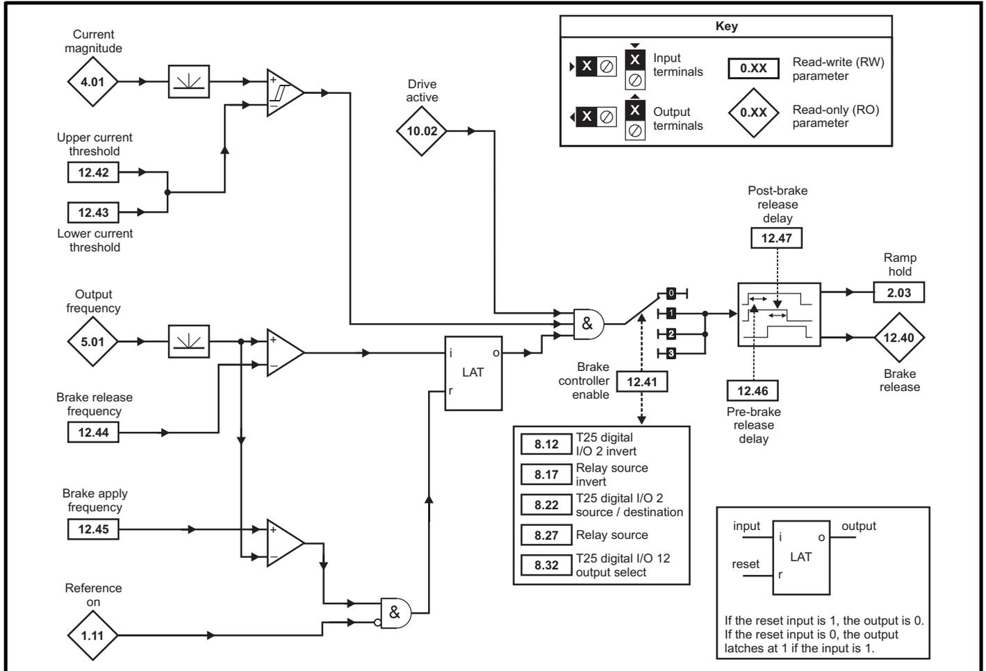
**Figure 13-17 Open-loop brake sequence**
