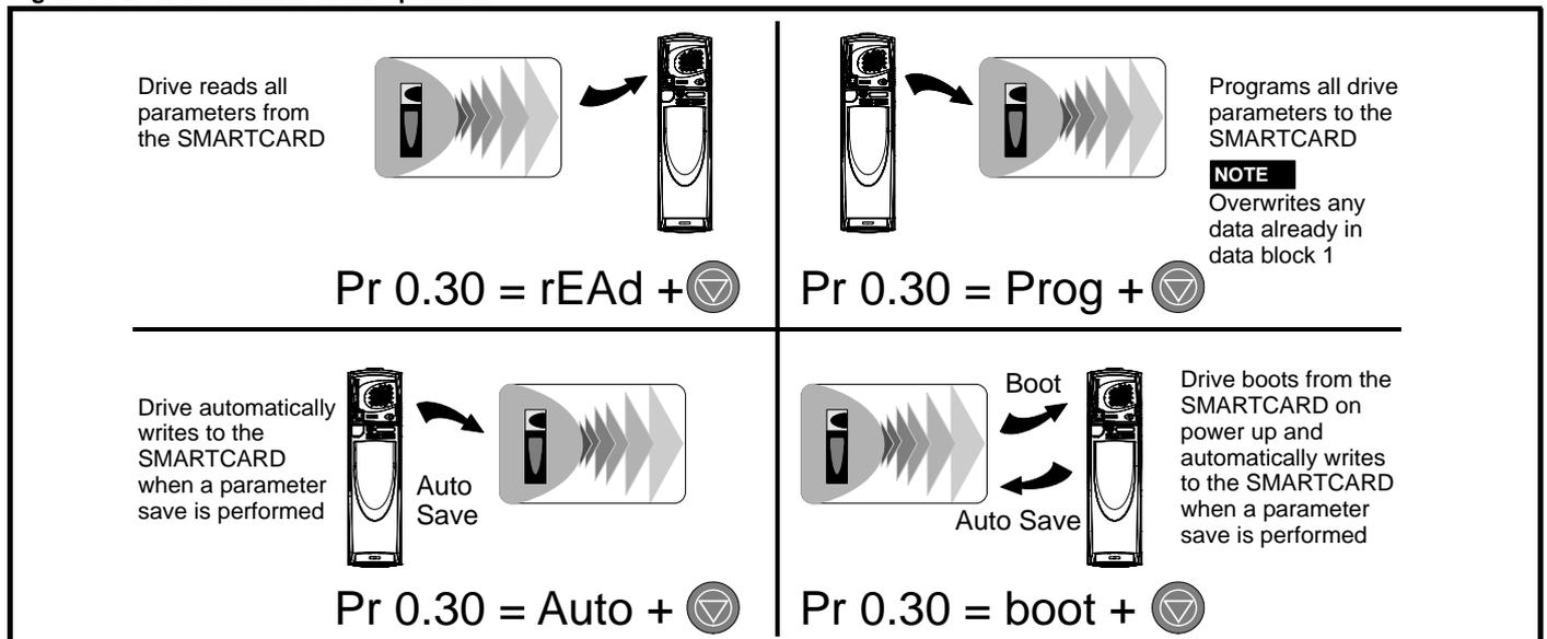
The SMARTCARD has 999 individual data block locations. Each individual location from 1 to 499 can be used to store data until the capacity of the SMARTCARD is used. With software V01.07.00 and later the drive can support SMARTCARDS with a capacity of between 4kB and 512kB. With software V01.06.02 and earlier the drive can support SMARTCARDS with a capacity of 4kB.
