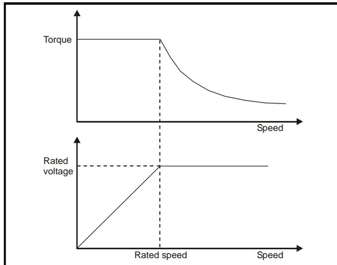
Care must be taken to ensure the torque available above base speed is sufficient for the application to run satisfactorily.
