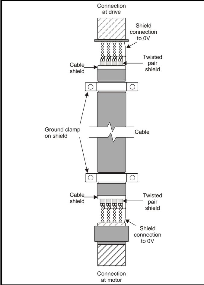
**To ensure suppression of radio frequency emission, observe the following:**
