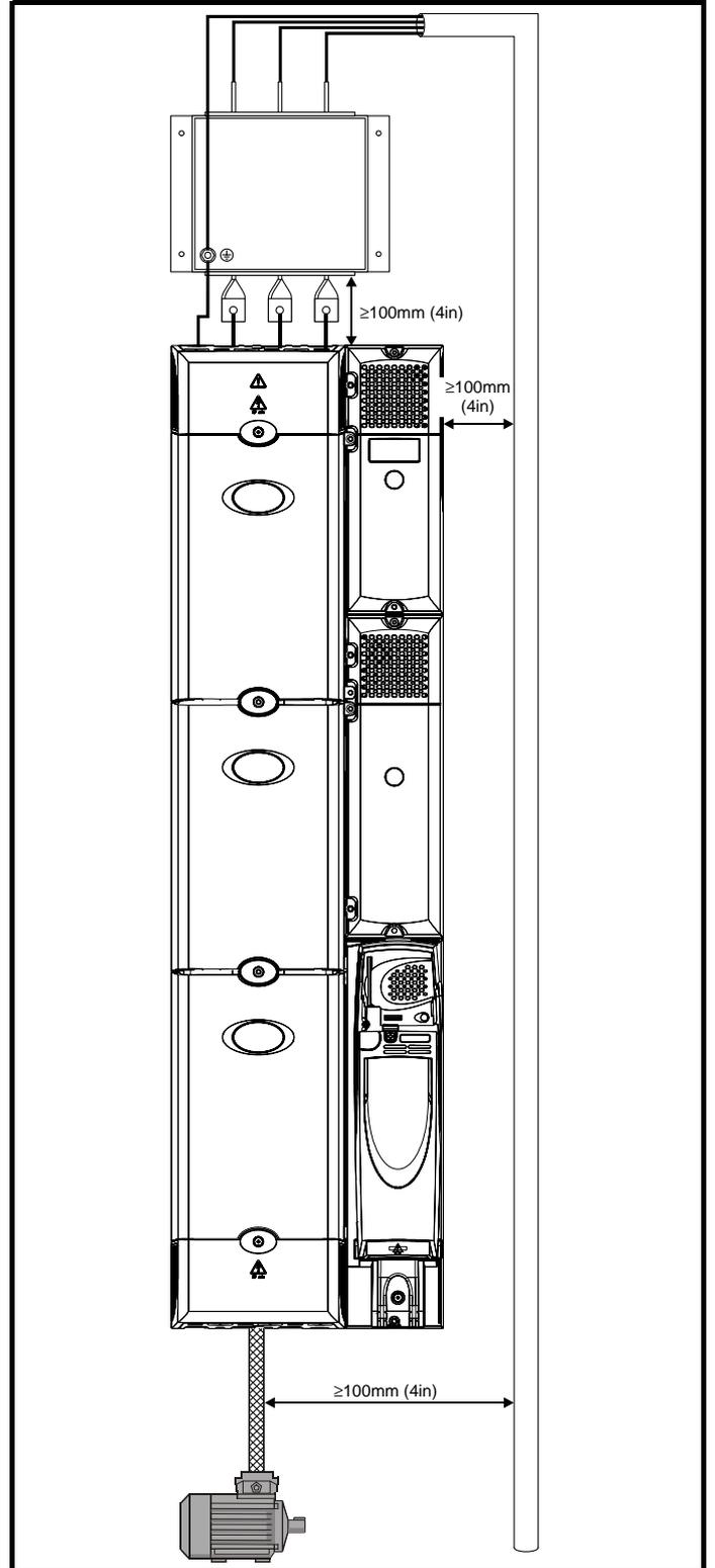
Avoid placing sensitive signal circuits in a zone 300mm (12in) all around the power module.
