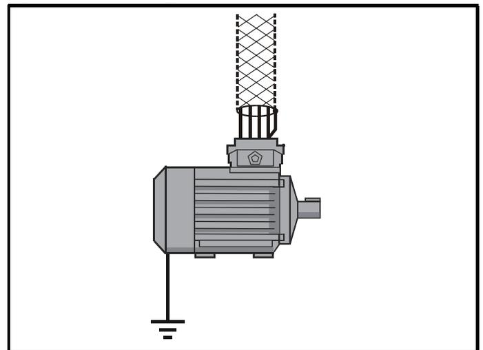
Unshielded wiring to the optional braking resistor(s) may be used, provided the wiring does not run external to the enclosure. Ensure a minimum spacing of 300mm (12in) from signal wiring and the AC supply wiring to the external EMC filter. Otherwise this wiring must be shielded.
