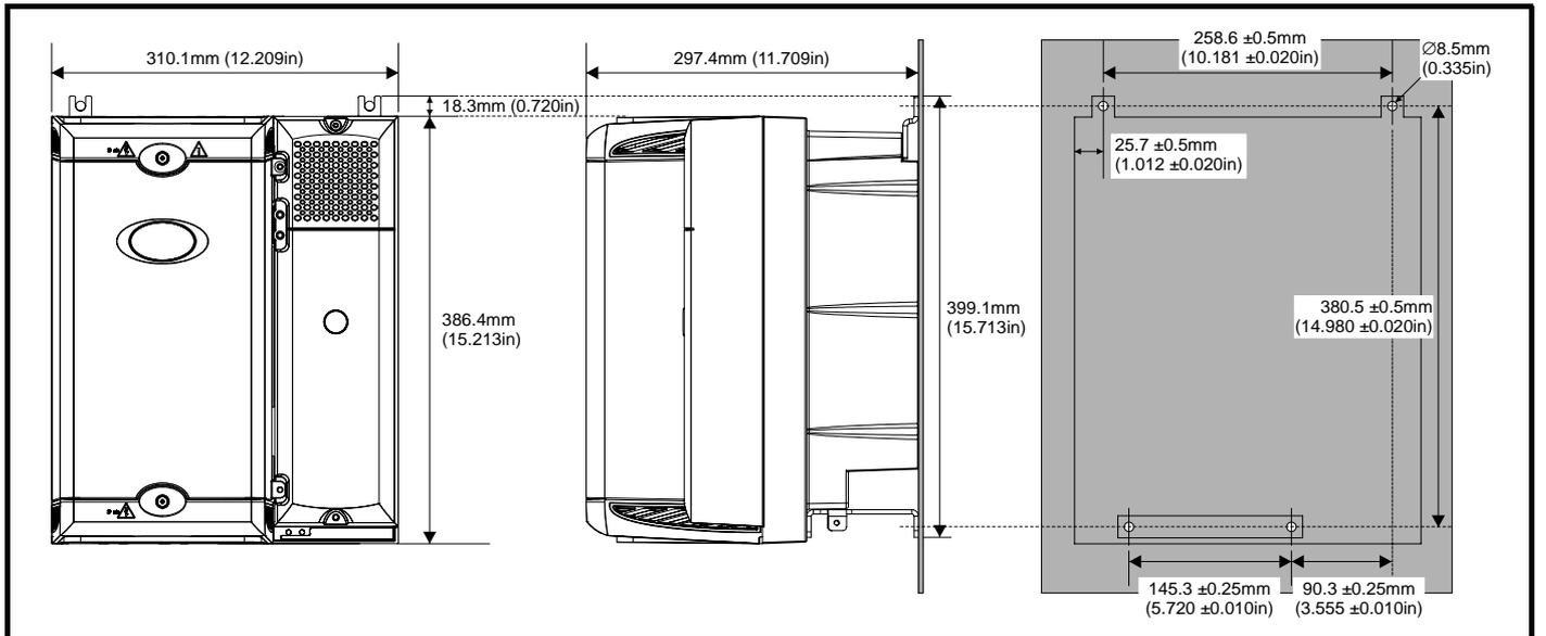
**Figure 5-10 Surface mounting the Unidrive SPMD with SPMC/U (rectifier) and docking kit**
