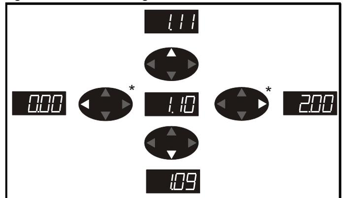
\* can only be used to move between menus if L2 access has been enabled (Pr 0.49). Refer to section 7.9 *Parameter access level and security* on page 84.
