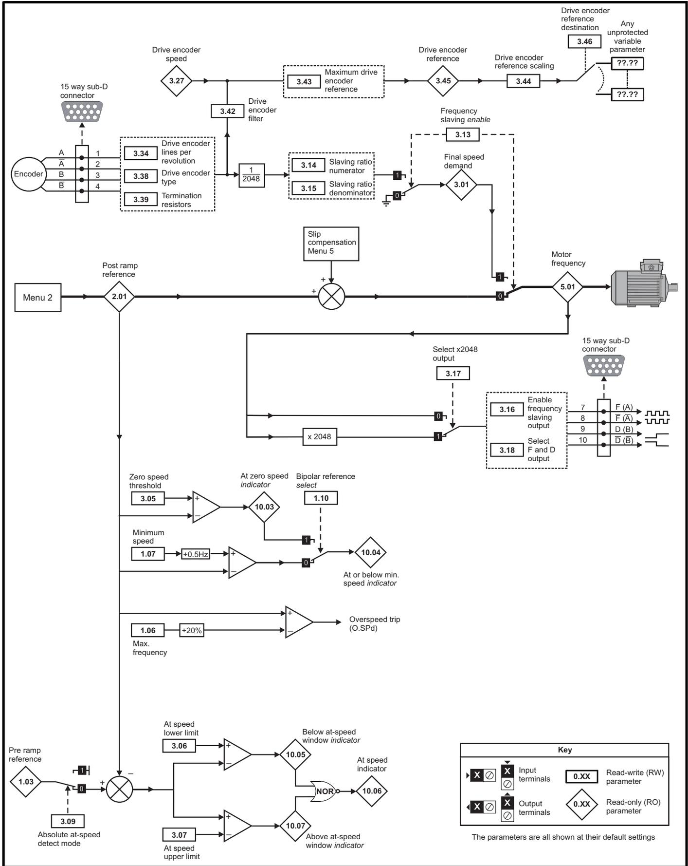
**Figure 13-4 Menu 3 Closed loop logic diagram**
