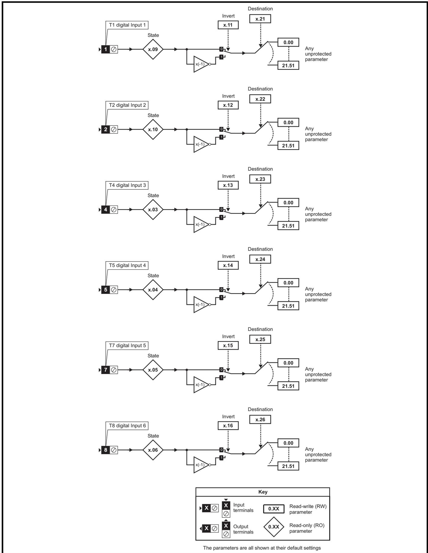
**Figure 13-39 SM-I/O 120V digital I/O logic diagram**
