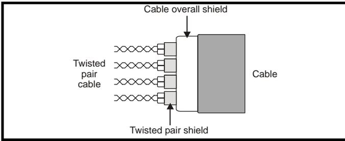
**Figure 6-19 Feedback cable connections**
