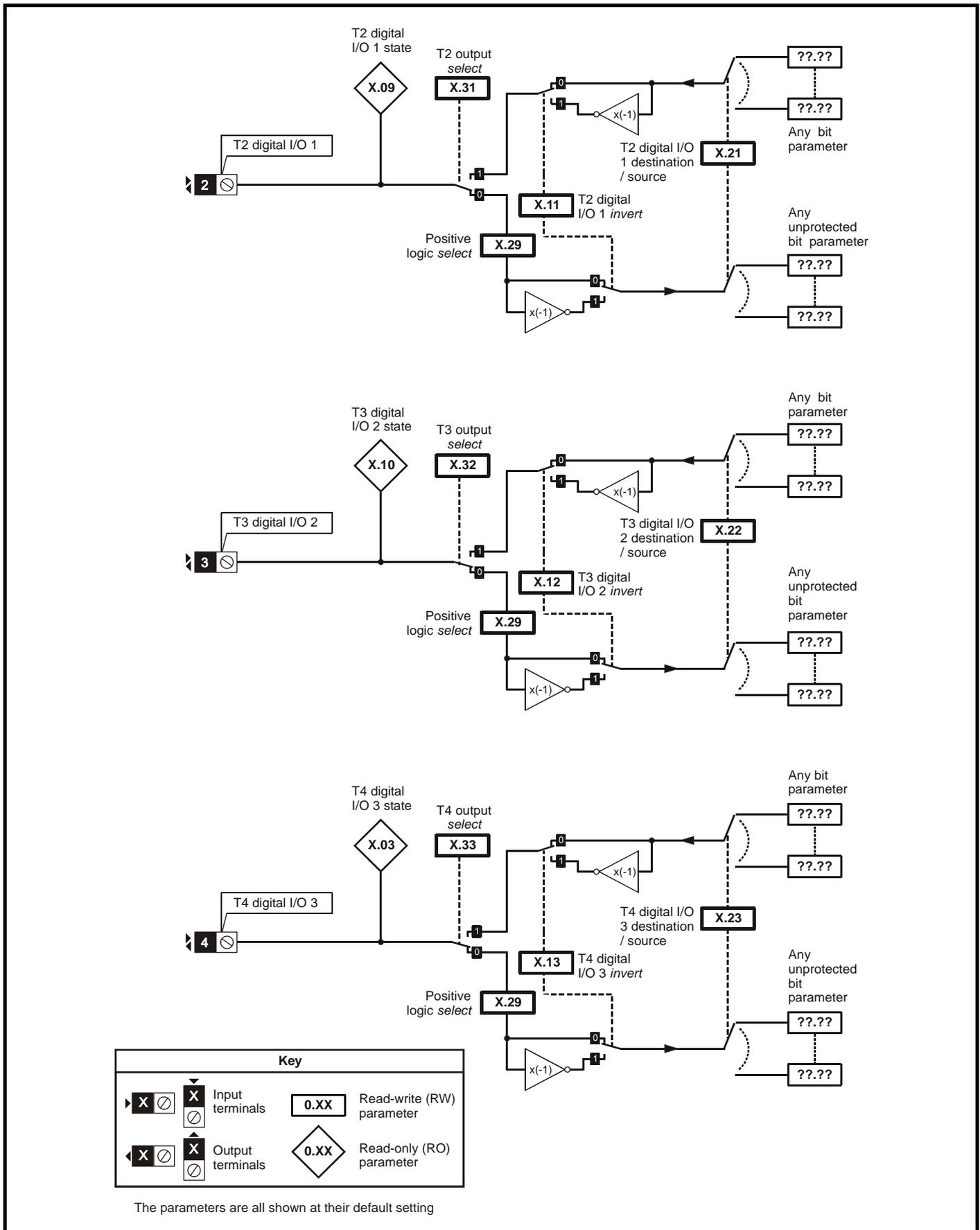
Figure 13-29 SM-I/O Plus digital logic diagram 2
