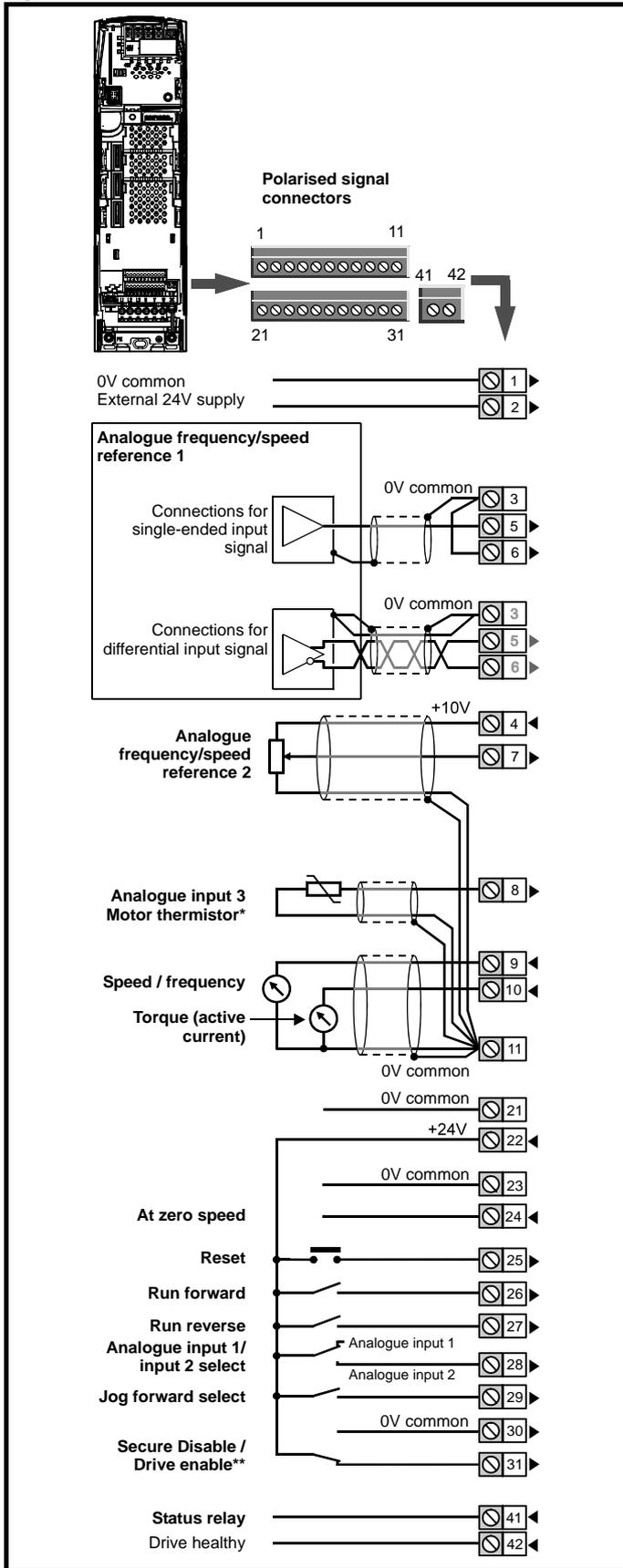
\* With software V01.07.00 and later, Analogue input 3 is configured as a motor thermistor input. With software V01.06.02 and earlier, Analogue input 3 has no default function. Refer to *Analogue input 3* on page 71.
