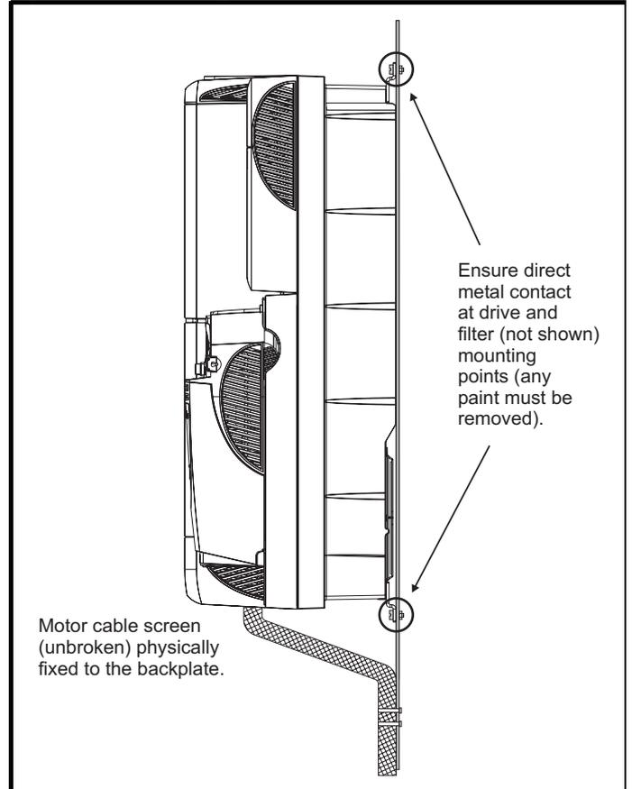
Connect the shield of the motor cable to the ground terminal of the motor frame using a link that is as short as possible and not exceeding 50mm (2in) long. A full 360° termination of the shield to the terminal housing of the motor is beneficial.
