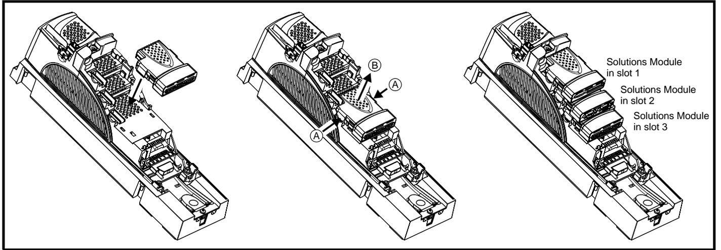
To fit the Solutions Module, press down in the direction shown above until it clicks into place.
