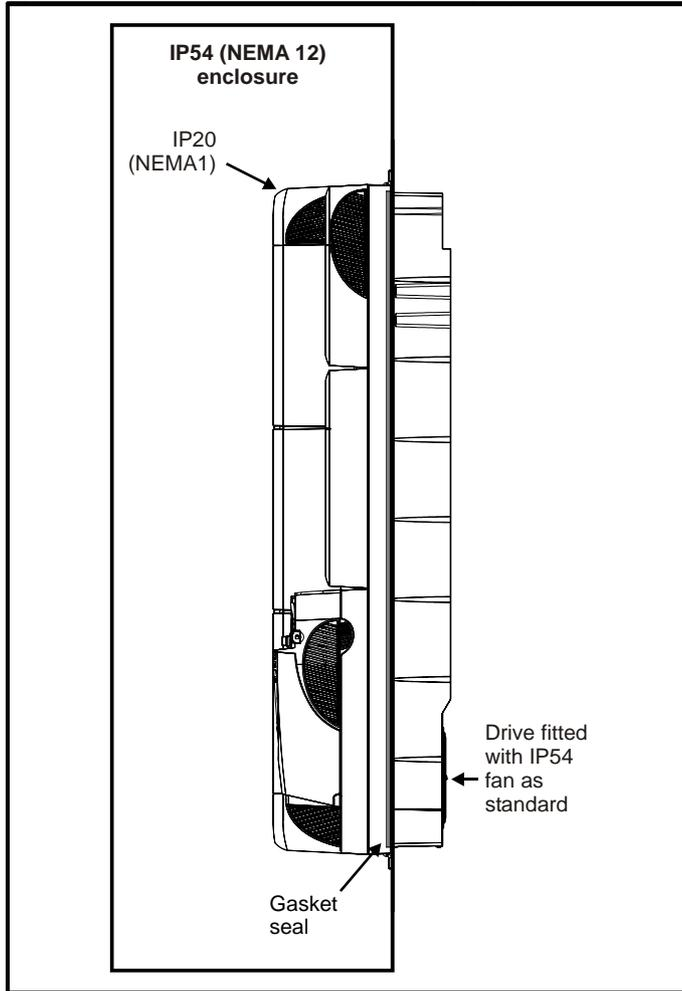
The heatsink fan fitted to Unidrive SPMA and SPMD are IP54 rated as standard.
