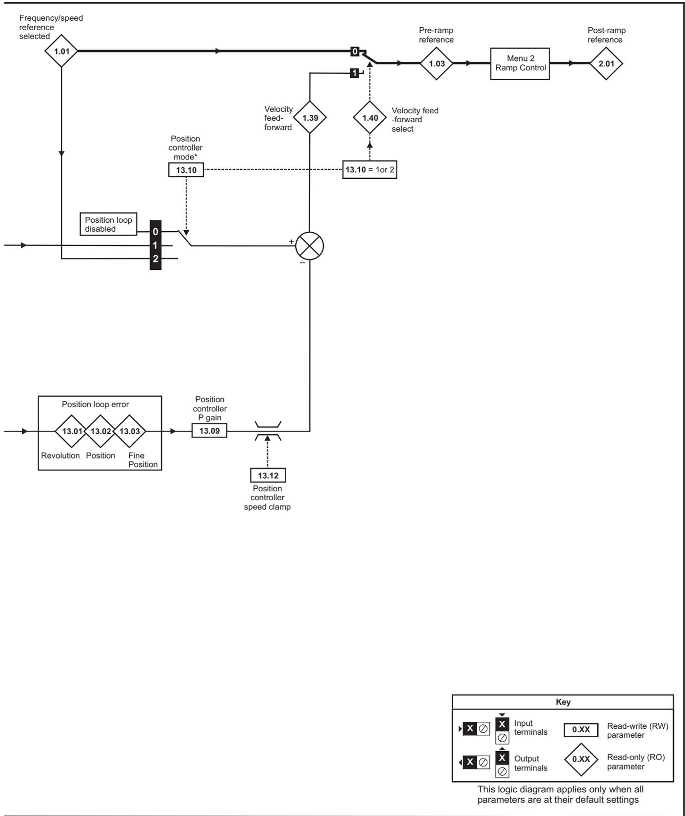
Figure 13-21 Menu 13 Closed-loop logic diagram
