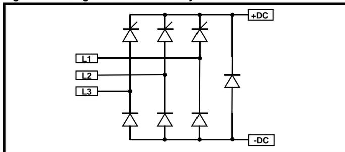
Figure 2-2 Dual half controlled thyristor
