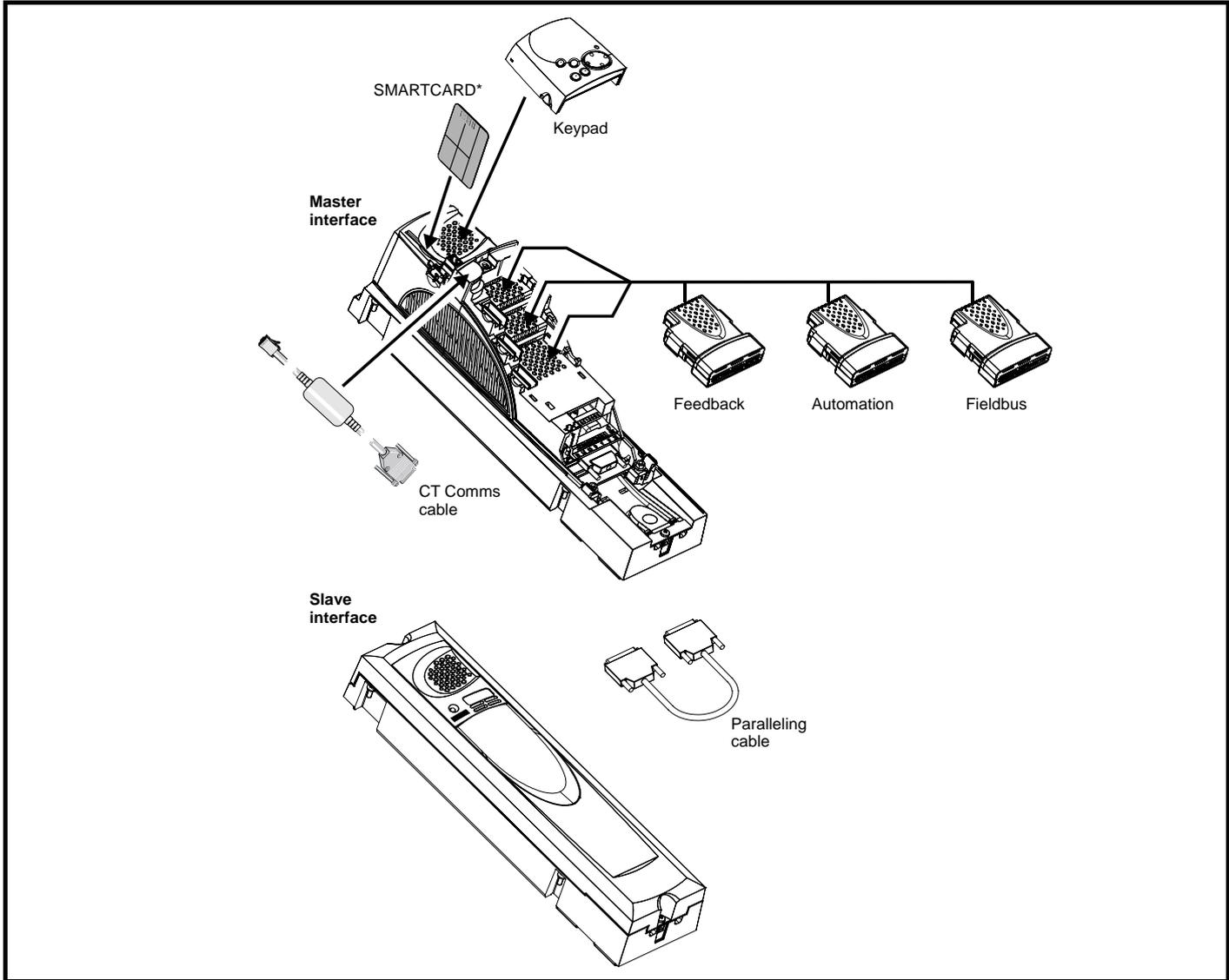
\* A SMARTCARD is provided with the Unidrive SPMA and SPMD master modules as standard. Only one SMARTCARD can be fitted at any one time. For further information, refer to Chapter 11 SMARTCARD operation on page 127.
