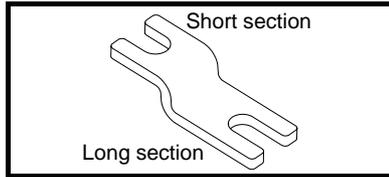
The mounting bracket must be fitted in the correct orientation with the long section inserted into or attached to the drive and the short section attached to the back plate. Figure 5-16 shows the orientation of the mounting bracket when the drive is surface and through-panel mounted.
