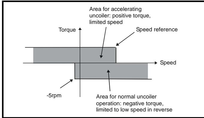
**4: Speed control with torque feed-forward**
