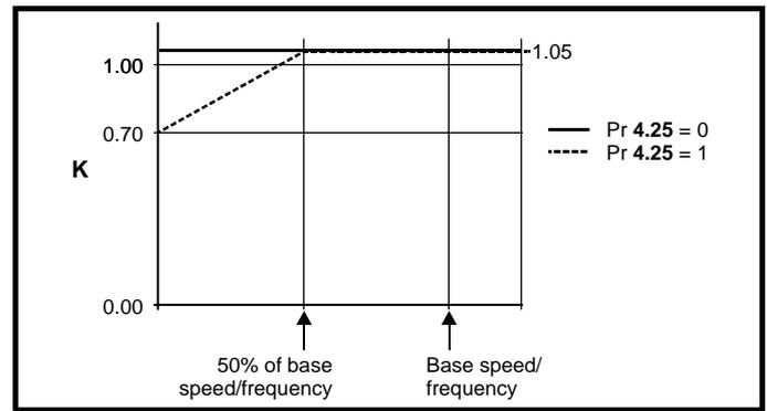
If Pr 4.25 is 0 the characteristic is for a motor which can operate at rated current over the whole speed range. Induction motors with this type of characteristic normally have forced cooling. If Pr 4.25 is 1 the characteristic is intended for motors where the cooling effect of motor fan reduces with reduced motor speed below 50% of base speed/frequency. The maximum value for  $K$  is 1.05, so that above the knee of the characteristics the motor can operate continuously up to 1.05% current.
