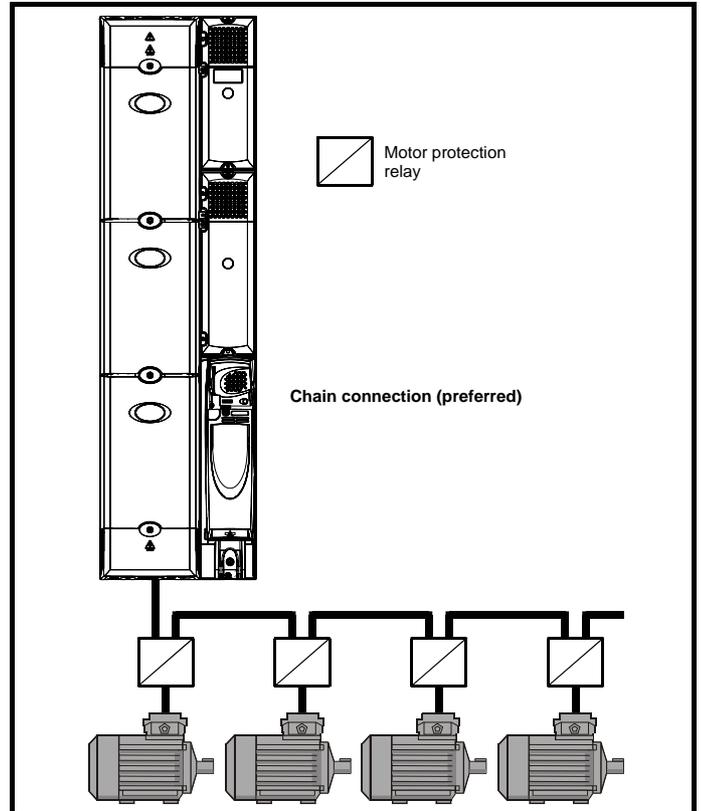
**Figure 6-12 Alternative connection for multiple motors**
